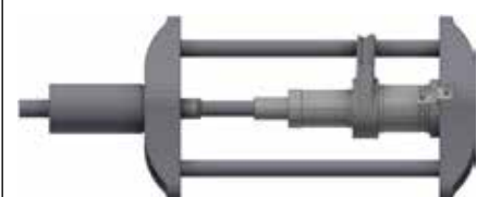
Installation situation of a slotted and tensioned bushing
