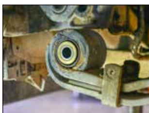
Installation situation of a slotted and tensioned bushing
